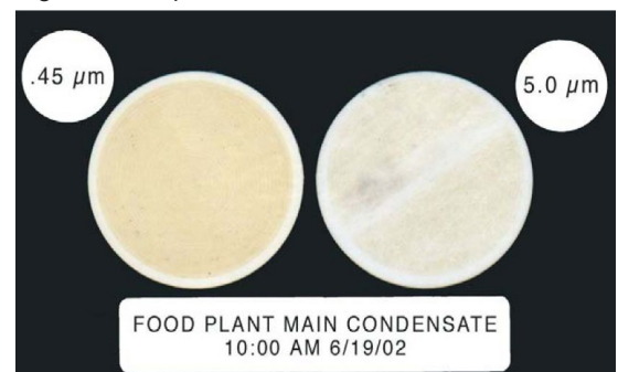
Figure 2: Millipore filter test results after BL1562
