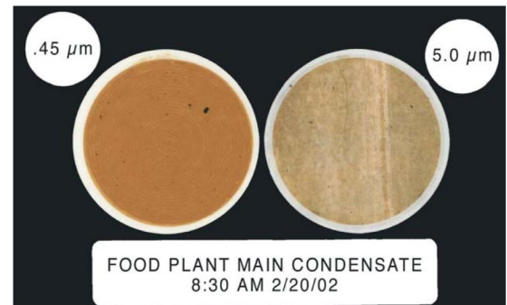
Figure 1: Millipore filter test results before BL1562
