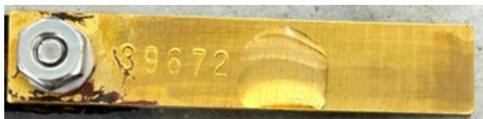
A brass corrosion coupon treated with MultiCuRE exhibits hydrophobicity, with water beading on the surface to inhibit corrosion.
