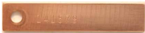
Copper corrosion coupon after FlexGuard application Corrosion rate <0.1 mpy
