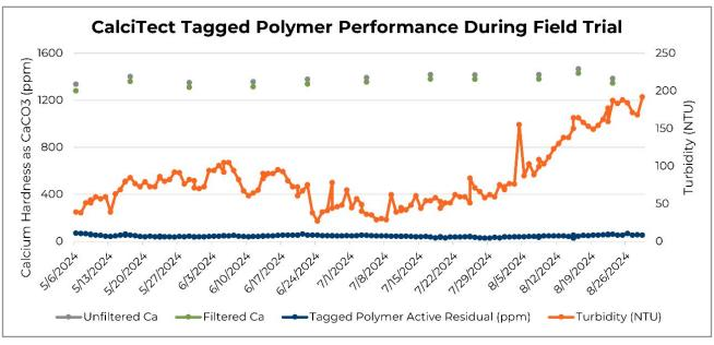
Performance of the non-phosphorous, tagged polymer in CalciTect with high-turbidity makeup water application. The minimal difference between filtered and unfiltered calcium hardness indicates the product's ability to manage scale deposition during the entire field trial.
