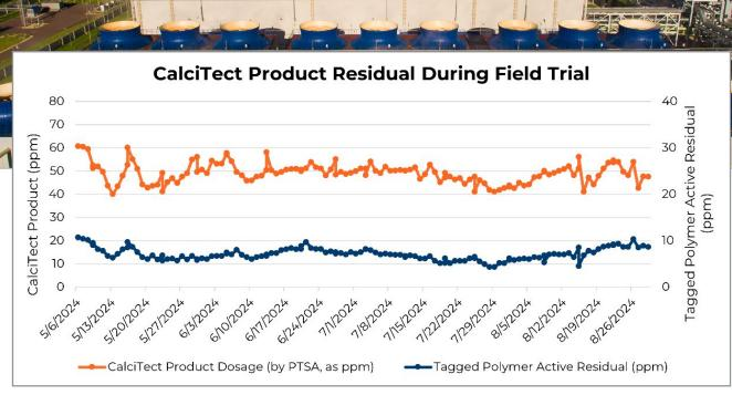
Monitoring of CalciTect product (by PTSA) and active polymer residual (by tag) shows consistent dosing throughout several months of the field trial.
