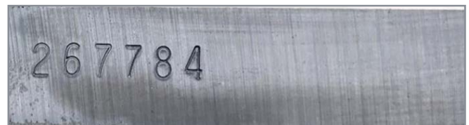
Mild Steel Coupon After FlexCorr Trial
