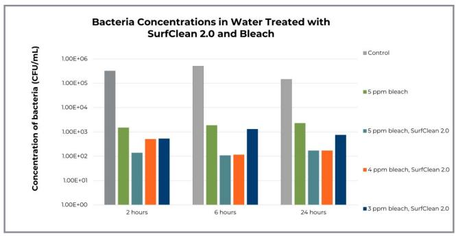
This chart shows sessile bacteria levels in untreated cooling water versus four variations of treatment.
