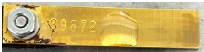
Corrosion coupon showing the hydrophobic film formed by MultiCuRE
