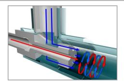
The custom-designed Tempest hydro-kinetic disperser tee enables the system to provide the right type of mixing energy at the crucial moment of initial wetting and taper that energy through a multi-stage hydration regime. The result is a fully hydrated polymer solution with maximum charge site exposure, helping optimize polymer usage and performance.
