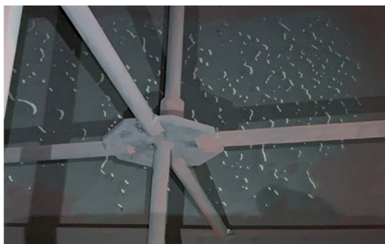
Tiger stripe pattern indicating two-phase flow-accelerated corrosion prior to FFA treatment
