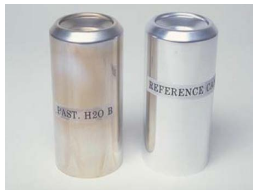
Figure 1: The can on the left demonstrates the appearance of magnesium silicate on the unprotected surface of the can, compared to a reference can with no staining.
