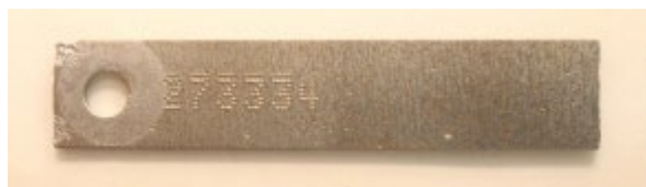
ChemTreat's mild steel treatment program achieved a corrosion rate of 1.4 mpy after a 90-day trial.
