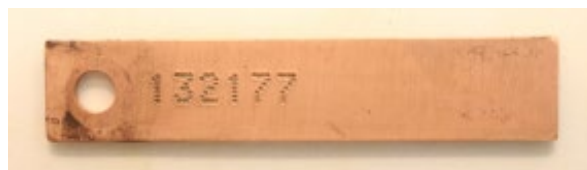
ChemTreat's copper corrosion treatment program achieved a corrosion rate of 0.9 mpy after a 90-day trial.
