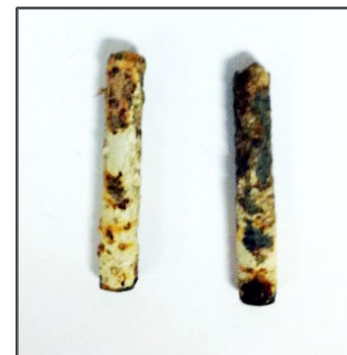
16 Stork - Corrater Tips - 05/20/14 Treated with phosphate NSF in system for 60 days; tips show corrosion and deposition
