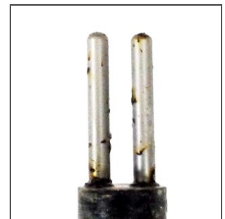
16 Stork - Corrater - 01/20/15 Treated with FlexPro® in system for 180 days (still in system); tips show minimal corrosion and no deposition
