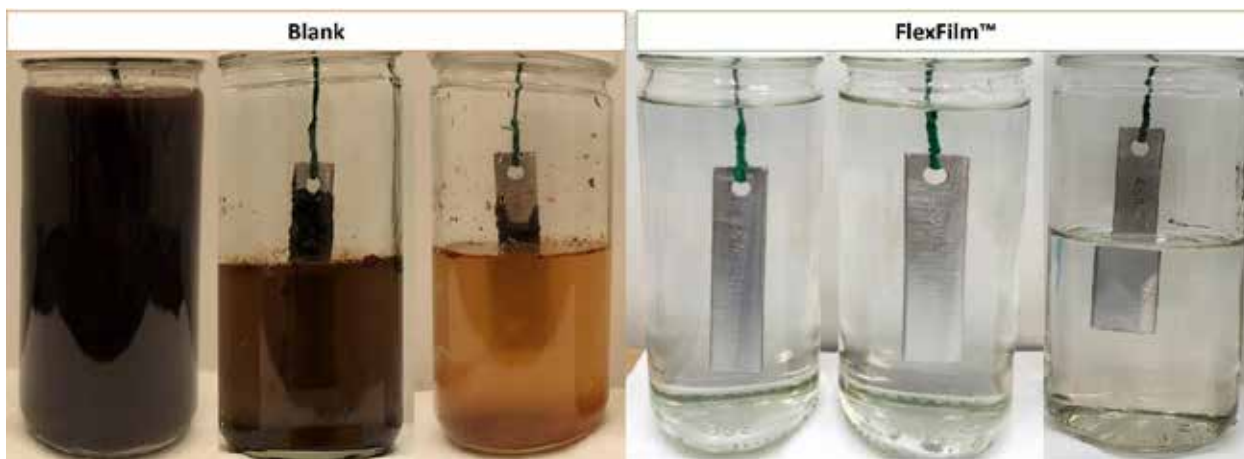
Blank and FlexFilm™ test results after 30 days
