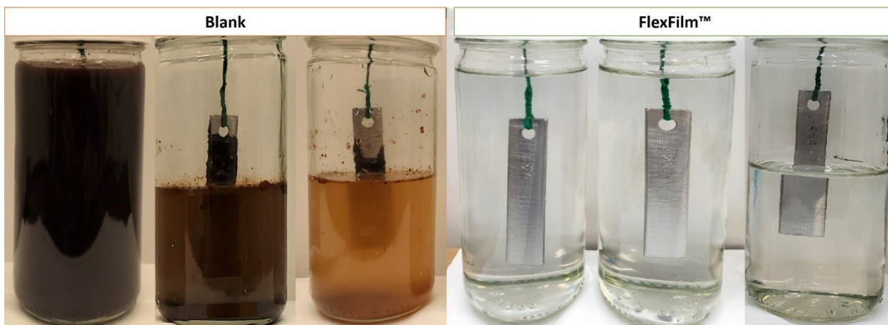
Blank and FlexFilm™ test results after 30 days
