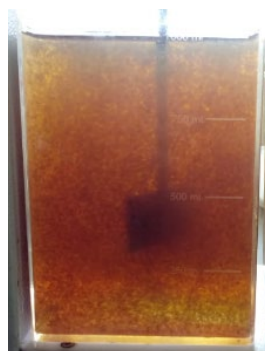
Jar test before P8200L application: low efficiency of floc formation, with light flocs of low density and low settling speed
