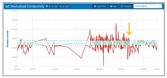
Neutralized conductivity trend chart generated by CTVista®+ to monitor performance. The green spectrum indicates the range of desired conductivity. The yellow arrow indicates when the new controller was installed.
