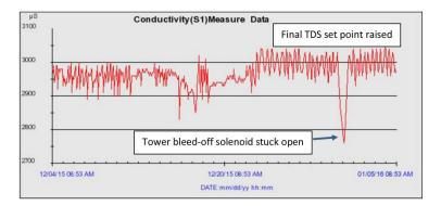
A tower operating at 4 versus 3 cycles will reduce water usage by 12%, inhibitor by 33%, saving approx. \$35,000 on acid, water, and treatment costs.
