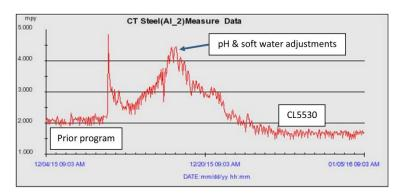
As shown in the graph on the left, once all of the system chemistries were set, corrosion rates eventually decreased from 2.1 to 1.6 mpy. Corrosion coupons are also being used to monitor program performance and have correlated very well with the on-line corrater readings.
