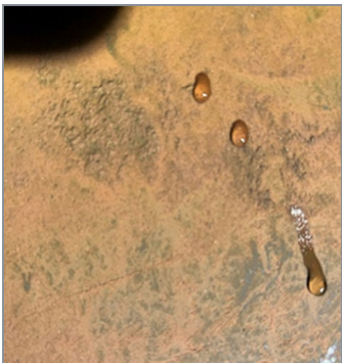
Water droplet formation on the drum shows that the FFA has passivated the surface with a hydrophobic layer
