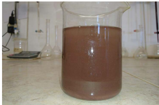
BEFORE: High turbidity in the overflow of the settling ponds
