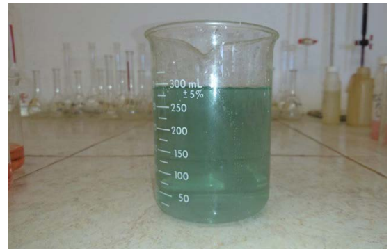
AFTER: Low turbidity in the overflow of the settling ponds
