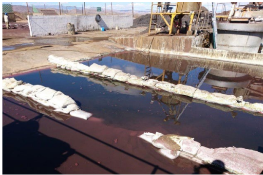
BEFORE: High turbidity in the settling ponds
