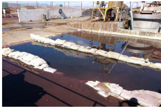
BEFORE: High turbidity in the settling ponds
