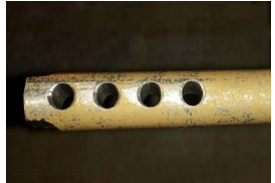
Coupon before treatment with ChemTreat ML708
