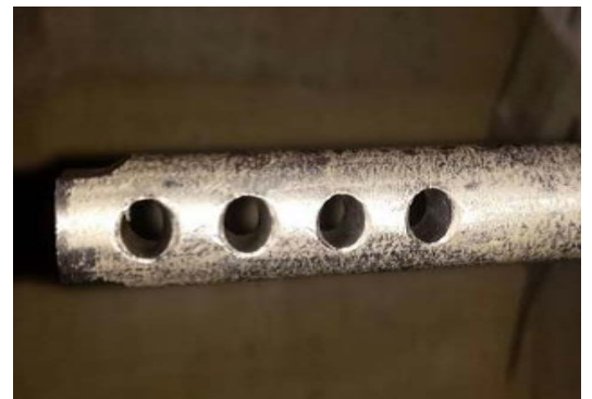
Coupon after treatment with ChemTreat ML708
