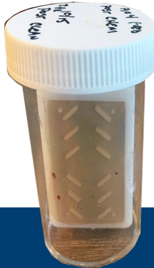
RO Makeup post-bisulfite feed and post-pipe cleaning
