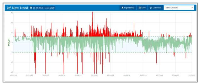
Trend charts showing pH and conductivity testing parameters increasingly staying within the acceptable range after CTVista®+ was fully adopted in April 2019. The shaded areas indicates the acceptable parameter range.
