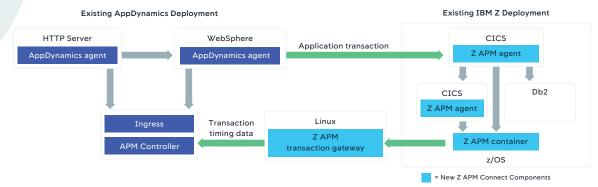
Required components: z/OS mainframe, IBM Z APM Connect license, AppDynamics Pro licenses, and a gateway box.
