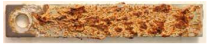
Before SurfClean 2.0 trial: mild steel coupon indicates severe system corrosion.
