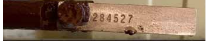
Two months into the SurfClean 2.0 trial: mild steel coupon shows significant corrosion reduction.
