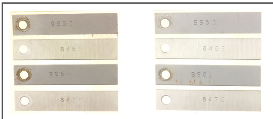
Before and after cleaning photos of mild steel and stainless steel corrosion coupons, FlexPro® Treatment
