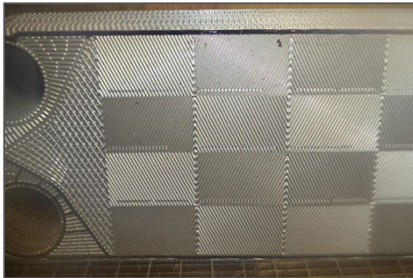
Plate and Frame Heat Exchanger Cooling Water Side with FlexPro® Treatment
