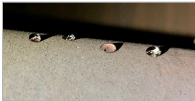
BL9000 protective film formation on the mild steel surface within the low-pressure steam drum.
