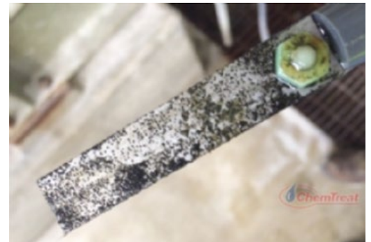
Elevated pitting corrosion in the untreated circuit.
