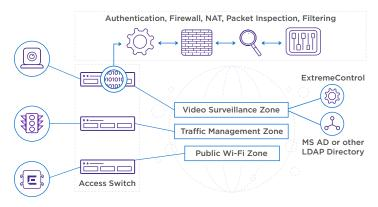
Figure 2: Segmented Zones for Smart City Functions
