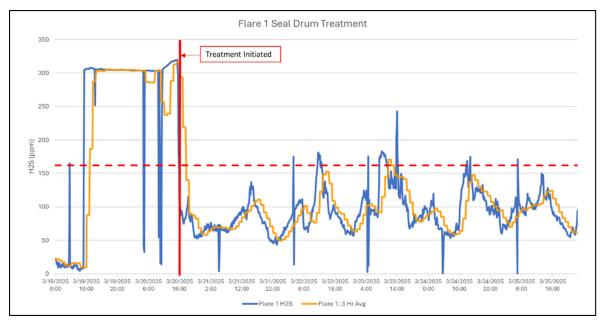
$H_2S$  levels were rapidly reduced in the flare 1 steam drum after CT9156 treatment was applied.
