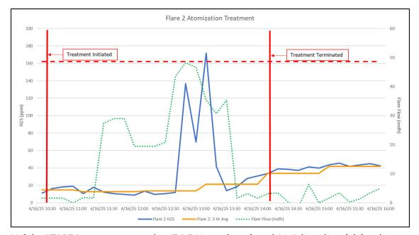
With CT9156 treatment, the FGRU maintained  $H_2S$  levels within the target range during a live flare job.
