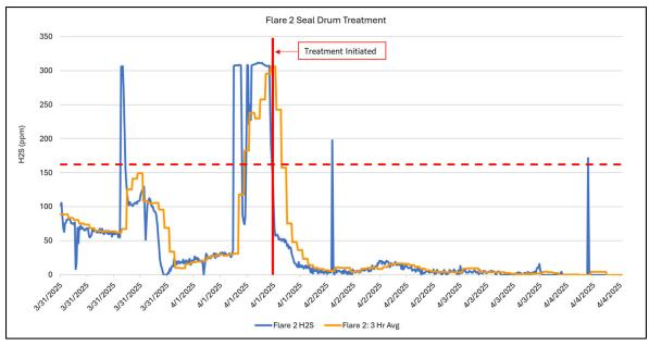
The flare 2 seal drum also saw a rapid reduction in  $H_2S$  load after CT9156 treatment.
