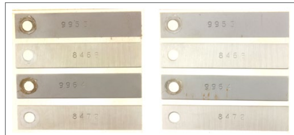
Corrosion coupons downstream of the heat exchanger show results before and after cleaning.
