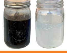
Example of frac recycle water before and after polymer application. Approximately 6 ppm of neat polymer was needed to pull the solids out of solution
