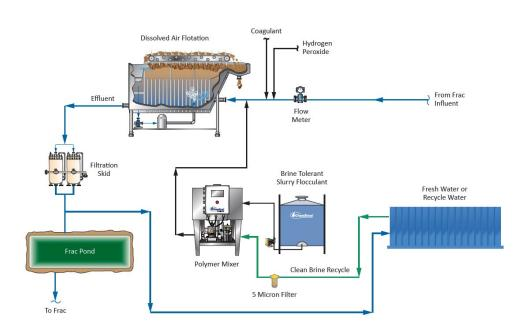
Example of brine-tolerant slurry flocculant (highly flocculating polymer) application at a hydraulic fracturing site.
