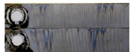
FlexCorr (Mild Steel) Average Corrosion rate: 1.60 mpy
