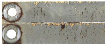
Blank (Mild Steel) Average Corrosion rate: 3.41 mpy
