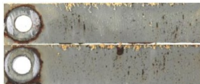
Blank (Mild Steel) Average Corrosion rate: 3.41 mpy
