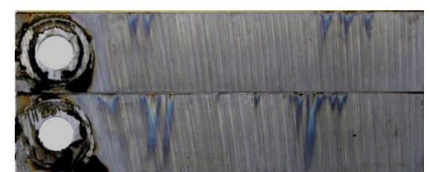
FlexCorr (Mild Steel) Average Corrosion rate: 1.60 mpy
