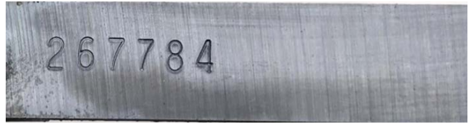
Mild Steel Coupon After FlexCorr Trial
