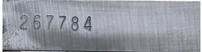
Mild Steel Coupon After FlexCorr Trial
